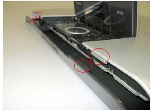
2) Remove the panel frame from the top cover (6 screws).
