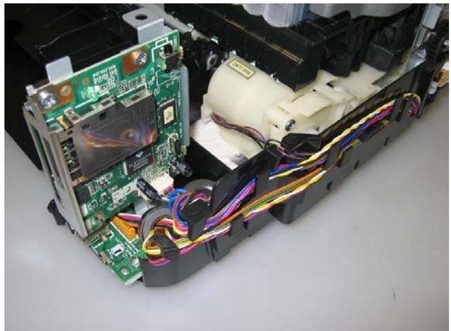
2) Seen from the back side of the machine (Note the DC harness position.)
