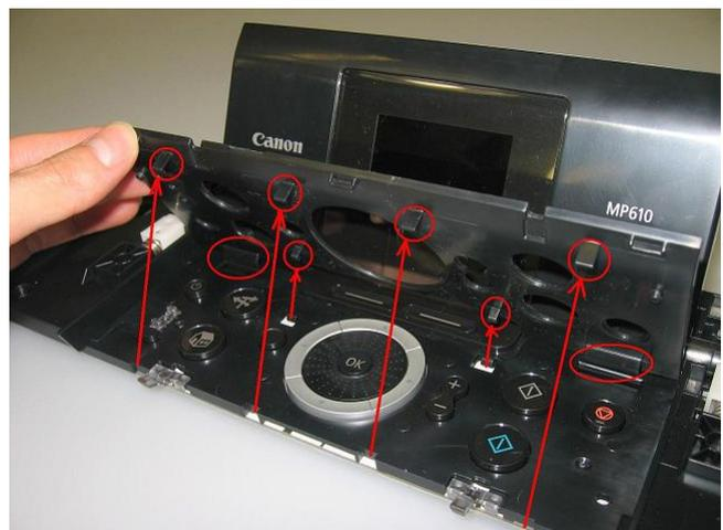
3) Remove the LCD and panel board from the panel frame.
