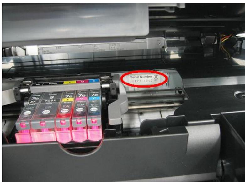
On the carriage flexible cable holder (visible on the right of the carriage after the machine is turned on, the scanning unit is opened, and the carriage stops at the ink tank replacement position)
