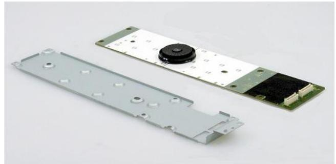
4) Remove the Easy-Scroll Wheel from the panel board.
